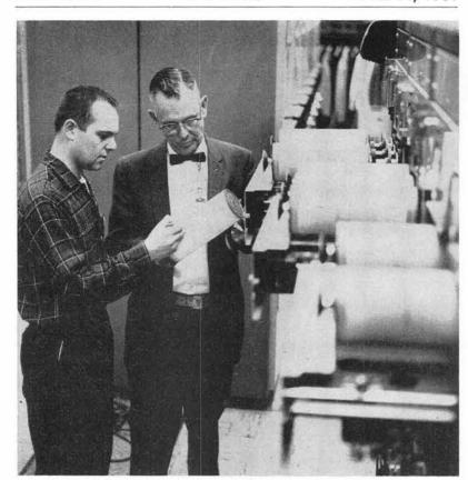
PROGRAMMING DRUMS control radiant heat facility tests. Test time, temperature, heat flow and power are represented as a line on the drum. Instruments "read" these lines. At left: D. F. McVey with A. R. Elwell. Tests rarely last more than 20 seconds.
